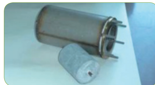
Figure 20: ATR catalyst and reactor
