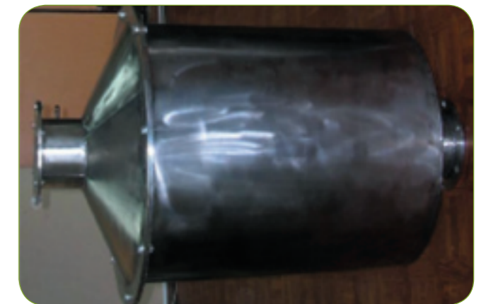
Figure 21: Radial-type DeNO x reactor
