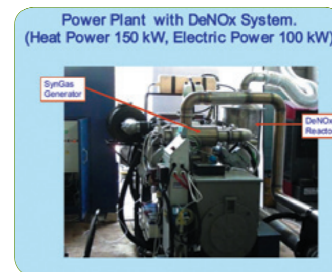
Figure 22: A system for NO x cleanup from exhaust gases
